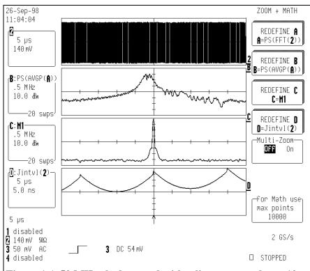
Figure 1 A 50 MHz clock spread with a linear ramp shows 10 dB reduction in peak spectrum level. JitterTrack of Interval error exhibits expected parabolic phase difference
